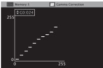
• On adjusting the brightness on the output side of bright parts on the disc side, the normally hard to see bright parts become clearly discernible images.
