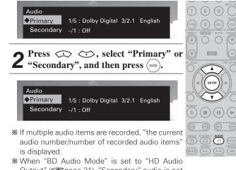
When "BD Audio Mode" is set to "HD Audio Output" (B page 31), "Secondary" audio is not output.
