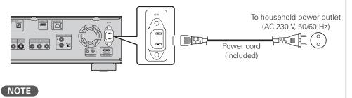
• Be sure to insert the power plug firmly. Incomplete connection results in noise generation.
