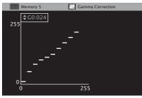
• On adjusting the brightness on the output side of dark parts on the disc side, the normally hard to see dark parts become clearly discernible images.
