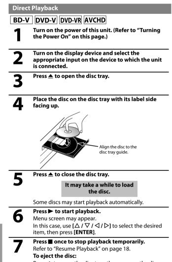
Press  $\triangleq$  to open the disc tray, then remove the disc before turning the unit to the standby mode.
