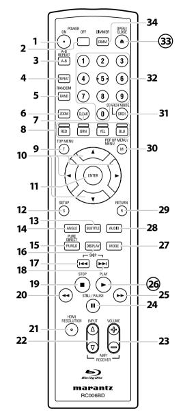
The unit can also be turned on by pressing the buttons with circled numbers.
